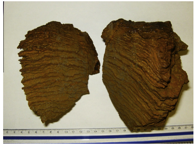
Fig. 4. Hand specimen of a hydrothermally laminated sample from the outcrop in Fig. 7. Centimeter ruler for scale.
